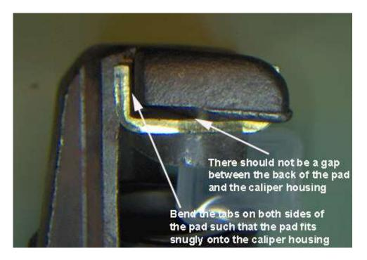
21. Apply a thin coating of grease to the bracket rails and the caliper keyways. Slip the caliper onto its bracket. Insure that the rails on the bracket seat onto the keyways on the caliper and that the brake pads are correctly positioned on each side of the rotor.
