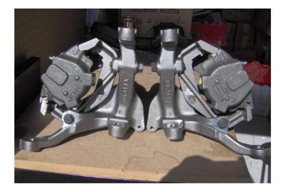
20. Place the outer pad into its place on the front inside of the caliper. Notice the tabs, on the pad, that wrap around the protrusion in the caliper. The tabs should be tapped with a hammer to make them fit tightly against the protrusion, but at the same time have the rear side of the pad flush against the front inside of the caliper. This fitting procedure will prevent rattling of the pad. You can also use a small amount pad adhesive seal on the rear of the pad to secure it to the caliper.
