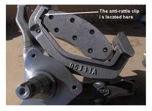
19. Select the caliper to mount. The part number for the right side is 4069 and the left is 4070. This is probably meaningless to you since you have most likely already removed the calipers from their boxes to admire them, and now have no idea which box they belong in. The caliper that results in the bleeder being in the forward higher position is the correct one. Note the position of the bleeder screws in the photo.
