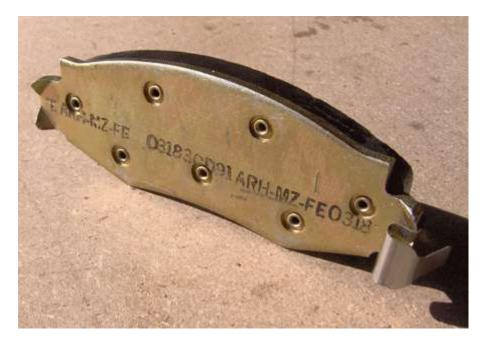
18. Turn the steering wheel to provide access to the inside of the caliper bracket. Insert the inner pad into its place, anti-rattle clip end first on the rearward end of the bracket. Press the pad's friction surface against the rotor. See the photo below for a guide to the pad orientation. The antirattle clip is located at the left side in the photo. THE CLIP AND PAD WILL FIT, BE PERSISTANT!
