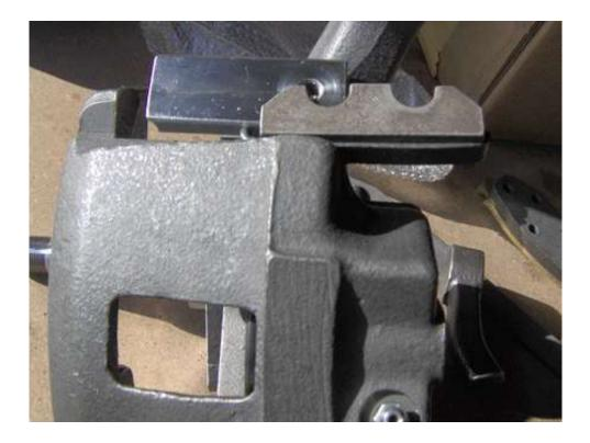
23. Hold the caliper in place and insert a support key-support key spring assembly. Use a hammer and carefully drive the support key assembly into place between the bracket rail and the caliper keyway. The key will seat <u>very</u> tightly. This is correct. See the photos below.
