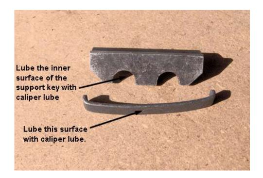
22. Apply a very thin layer of lube to the inner surface of the support key and the outer surface of the support key spring.
